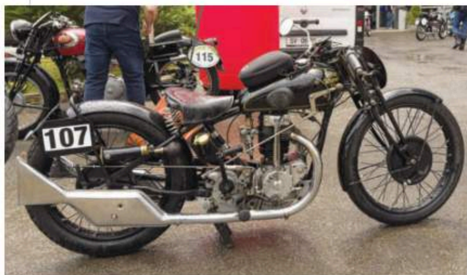
1929 Rudge Ulster with hand shift and Brooklands silencer — a rare sight!
